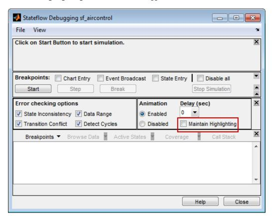
This enhancement enables you to inspect the active states of a chart after simulation ends, without having to use the SimState method highlightActiveStates. For more information, see Animating Stateflow Charts in the Stateflow User's Guide.
