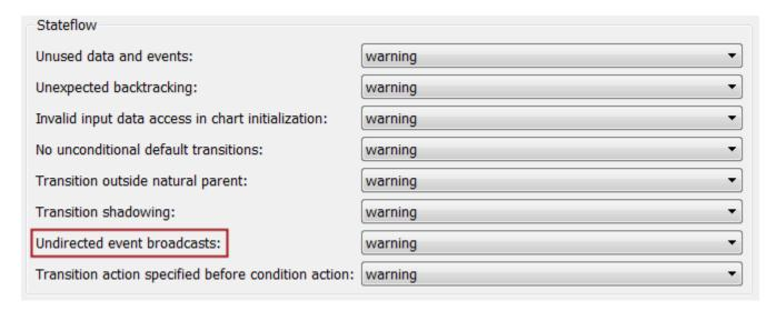
Undirected local event broadcasts can cause unwanted recursive behavior in a chart and inefficient code generation. You can avoid this behavior by using the send operator to create *directed* local event broadcasts. For more information, see Guidelines for Avoiding Unwanted Recursion in a Chart and Broadcasting Events to Synchronize States in the Stateflow documentation.
