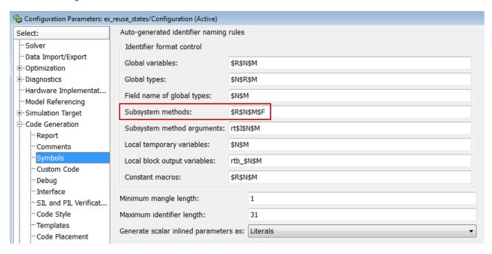
This enhancement enables you to control the format of generated function names for atomic subcharts when building an embedded real-time (ERT) target. For more information, see Generating Reusable Code for Unit Testing in the Stateflow User's Guide.
