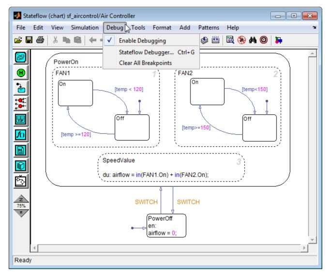
This enhancement enables you to focus on debugging a single chart, instead of having to debug all charts in the model. For details, see How to Enable Debugging for Charts in the Stateflow User's Guide.
