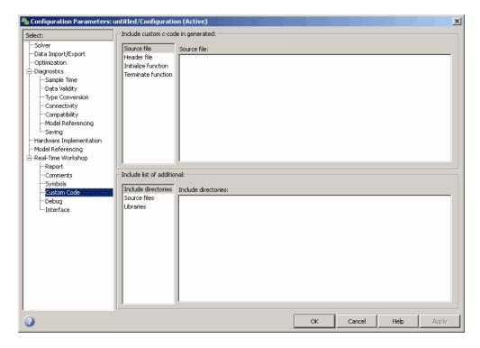
In R2008b, a new option is available in this pane: **Use the same custom code settings as Simulation Target**. You can use this option to copy the custom code settings from the **Simulation Target > Custom Code** pane to avoid entering the same information twice for the nonlibrary model.
